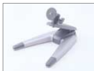
Monitor stand TW-MT1 A table-top stand for the monitor. Enables the monitor screen to be turned 180° to the left or right, and 90° upwards or downwards. Dimensions: 180 (width) x 100 to 170 (height) x 225 (depth) mm Weight: Approx. 530 g
