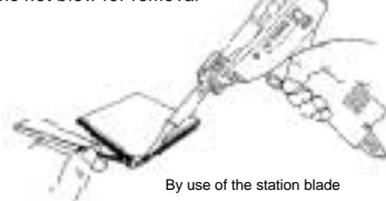
Melting the solder of other SMDs by the hot blow for removal
