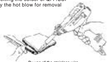
Melting the solder of QFP/SOP by the hot blow for removal
